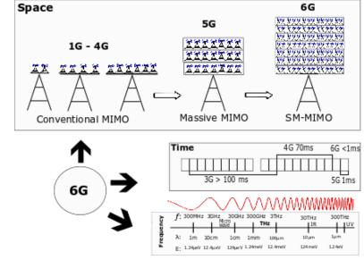
Fig. 1: An elucidation of resource utilization of 6G based on time-frequency space.
